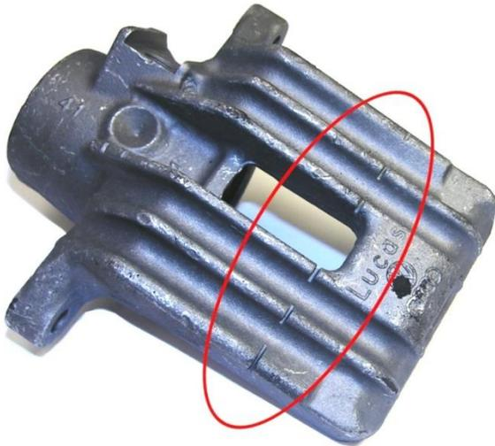
**Broken part / unauthorized repair / change in construction**
