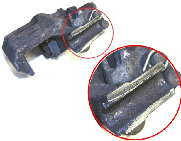
**Broken part / unauthorized repair**
