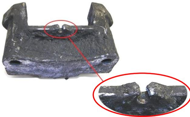
**Broken part / unauthorized repair**
