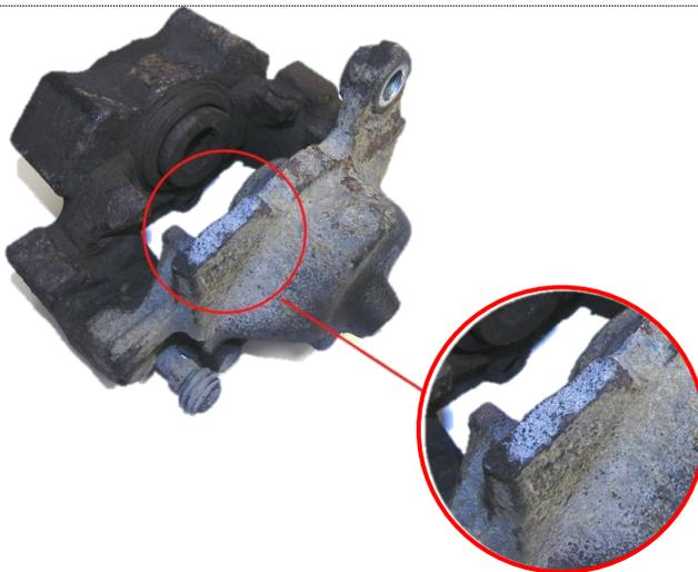
**Broken part / unauthorized repair**
