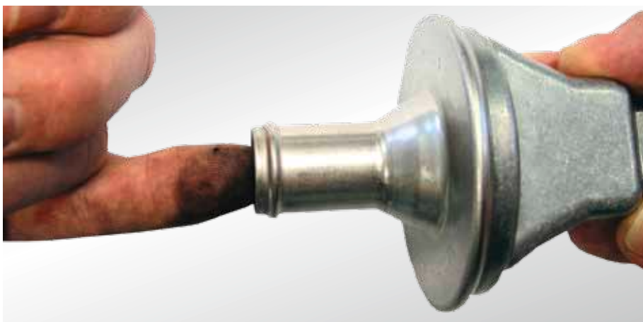
Simple inspection of the non-return valve
