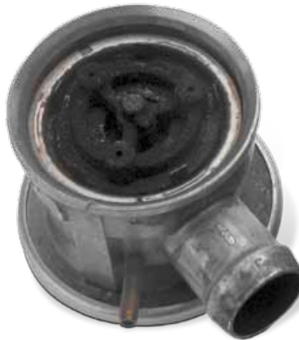
Damage as a result of exhaust gas condensate
