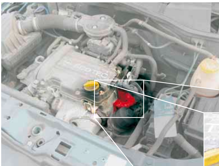
Electrical EGR-valve in the Opel Corsa (highlighted)
