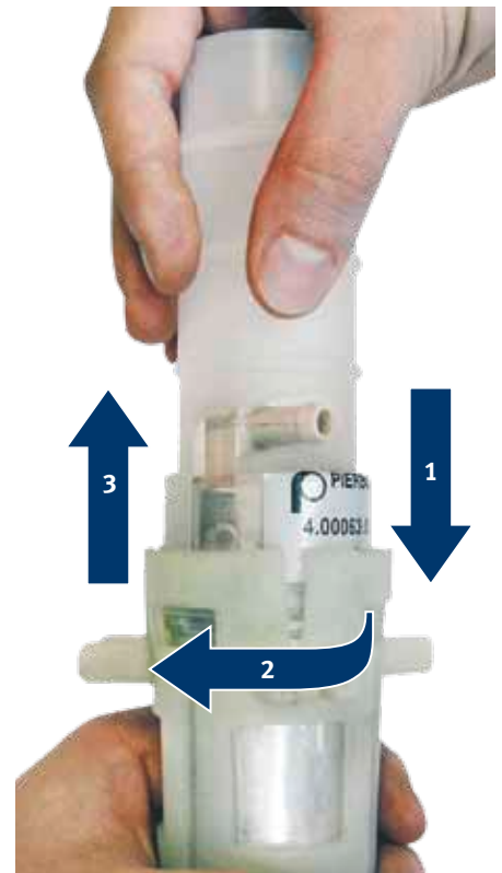
The tool expands the fixtures securing the fuel pump in the pump module. This functions extremely well on fuel pumps with an angled delivery-pipe tube.
