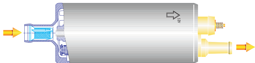
Suction intake of the prefilter
