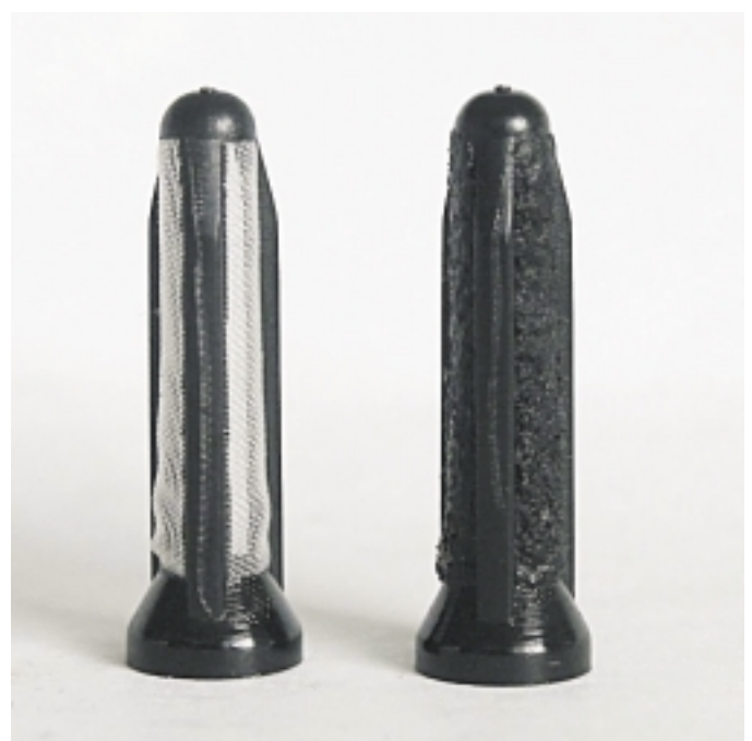
E1F Prefilters: - new (left), - clogged (right)
