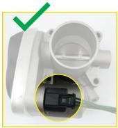
The female plug must snap firmly at the throttle body.
