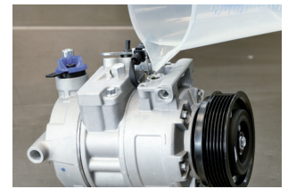
Figure 2: Pour the correct amount of oil for the system into the compressor and then reseal it.
