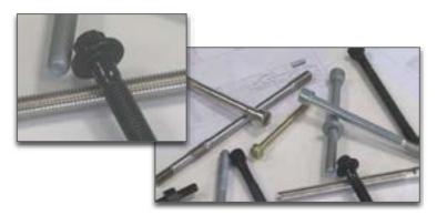
The main function of the cylinder head bolt is to apply the clamping force evenly across the different engine parts involved, usually cylinder block and head, with a capacity to hold it steady ensuring proper sealing of liquids and gases in the cylinder head gasket, withstanding temperature variations, vibrations and positional changes which occur in the engine during operation.
