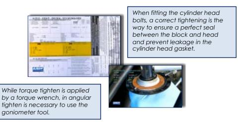
The bolt looseness involves insufficient clamping forces and therefore loss of liquids and gases in the cylinder head gasket, while if this is excessive the bolt will go too far trough the plastic zone it become to the breakage. In the same way, reuse cylinder head bolts with angular tighten can cause failure of the seal in the cylinder head and the bolt broken even suddenly before completing tightening.
