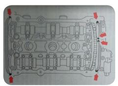
*NOTE:* To ensure the correct sealing of the cylinder head cover gasket, is absolutely necessary the application of this small quantity of silicone sealant over the mentioned transition areas.
