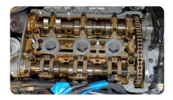
2. Apply sealant (Ajusil) in the transition area of the caps in the cylinder head as shown in the repair manual.
