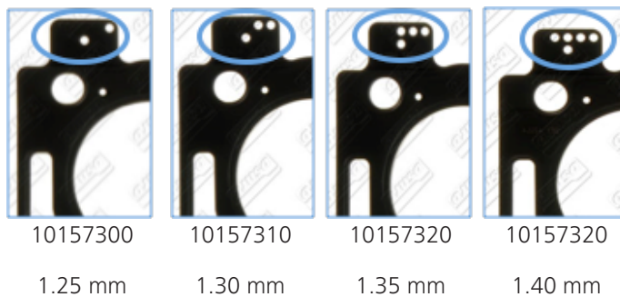
Examples of notches in head gaskets
