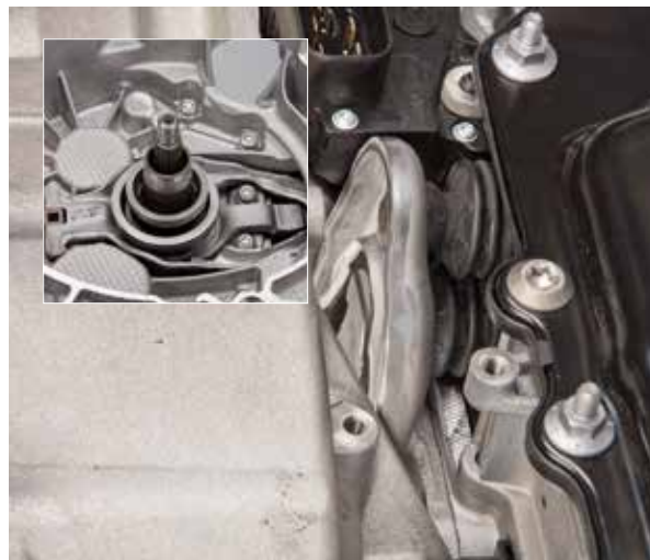
Engagement lever made from sheet steel – transmission construction date from June 2011, 2nd generation
